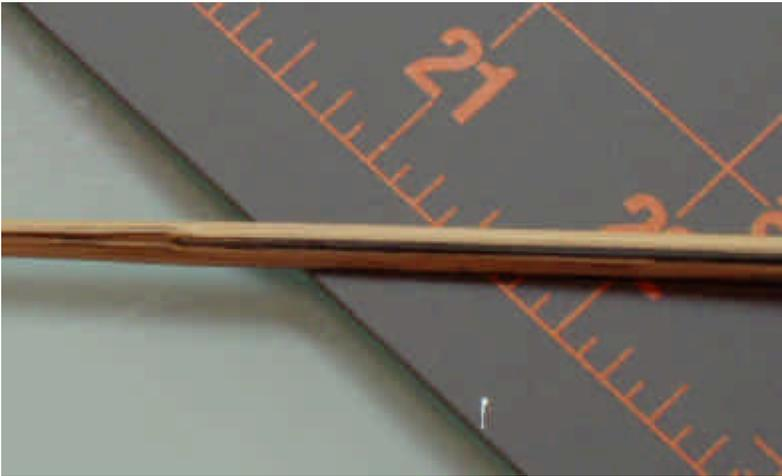
So far I really like the kite performance with this bamboo/carbon fiber combo-spine. There is one indirect aspect I also like about this spine arrangement. Even with a high wind kite; only one lower bridle connection is needed. Multiple bridle connection points along the spine are unnecessary. The carbon/bamboo laminated tail portion of the spine is so stiff that even with only one lower bridle connection point it has no tendency to flex backwards even in high winds.
