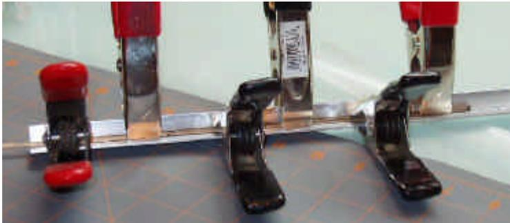
the tail portion of the spine as Mathias did, perpendicular to the skin side of the bamboo, **but before gluing and clamping the tail portion**, I first inserted a piece of flat carbon fiber into the split and then glued and clamped the two outer bamboo parts with the flat carbon sandwiched in between them. The size of carbon fiber I used is 0.019" thick x 0.118" wide; 0.48mm x 3mm. This is a very thin piece of flat carbon.
