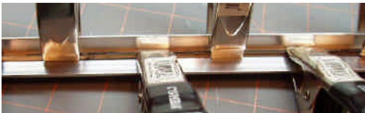
After the glue dries, I trim the carbon fiber so it's flush with the bamboo
