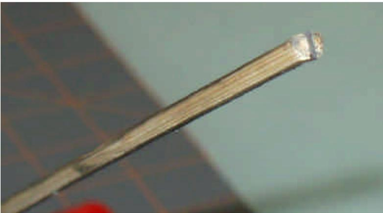
So far my experience is this spine provides a slightly faster kite. And one that tracks very well even out beyond the wind window edges. Its stiffness prevents virtually any wind energy being used in bending the lower portion of the spine backwards; instead all the energy from the wind is converted to energy used to push the kite forward.
