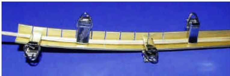
This 'jig' or 'form' allows Mathias to clamp the nose portion of the spine into a bend of his choice that is parallel to the skin side of the bamboo and also allows him to use the same form to clamp the laminated tail portion to be straight. However, the straight tail portion of the spine Mathias split **perpendicular** to the skin of the bamboo and clamped it to the vertical edge of his 'angled aluminum form'.
